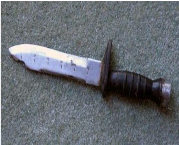
Contrary to the popular Hollywood image, the diver's knife has limited usefulness in fighting marauding sharks. It is, however, an essential item of safety equipment which can be used to cut the diver free from entanglements such as rope, kelp, fishing lines and nets. Scissors may be more effective for this.
