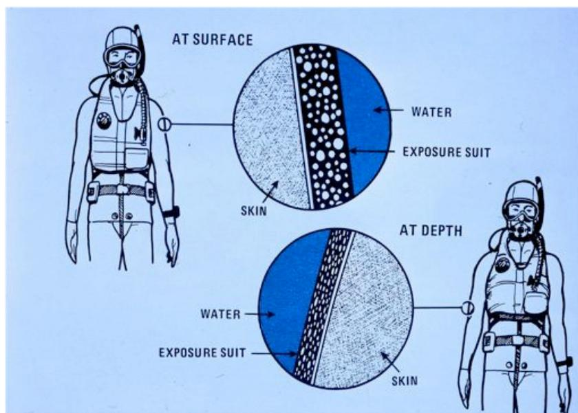
A poorly fitting wet suit can cause chafing, especially around the neck and arm-pit. A wet suit with an excessively tight neck can also compress the blood vessels to the brain leading to dizziness and fainting. Tightness around the chest may cause difficulty in breathing. Zippers allow for easier access and exit, but contribute to water leakage and reduced thermal reliability.
